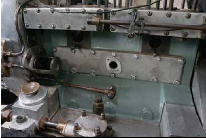
The engine block after repairs, and new side plate
