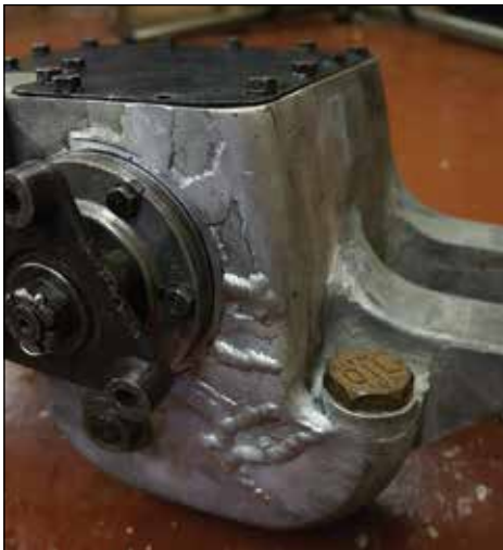
The repaired gearbox. Some extensive aluminium welding has taken place.
