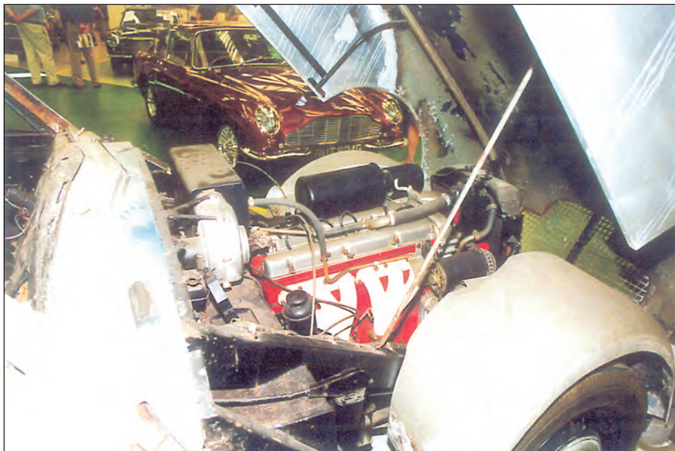
The Blue Monster. The whole front end lifts for maintenance, but 'mudguards' stay put so that dirt from tyres doesn't get on clothing. The engine is a standard LB6 (LB6A/50/220).
