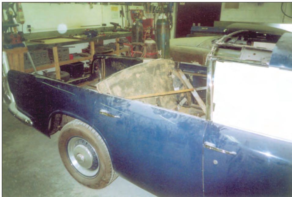
The old roof cut off ready for the new.
