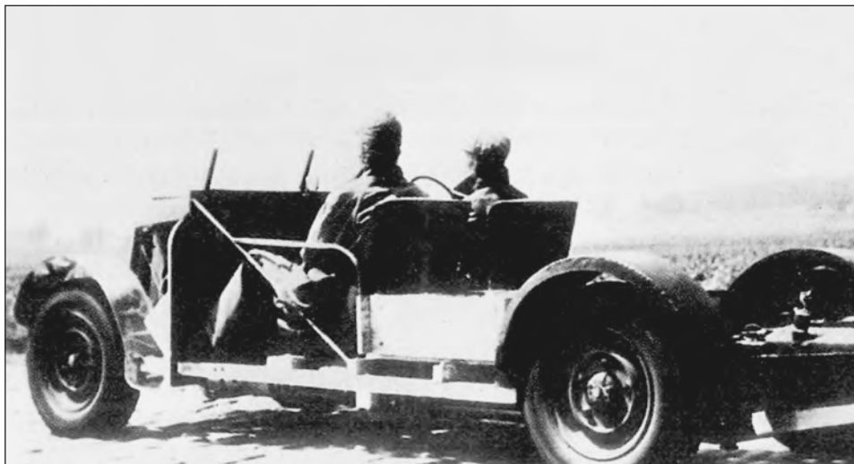
1953 picture of DP117 on test as a bare chassis with a 3 litre engine installed pro tem.
