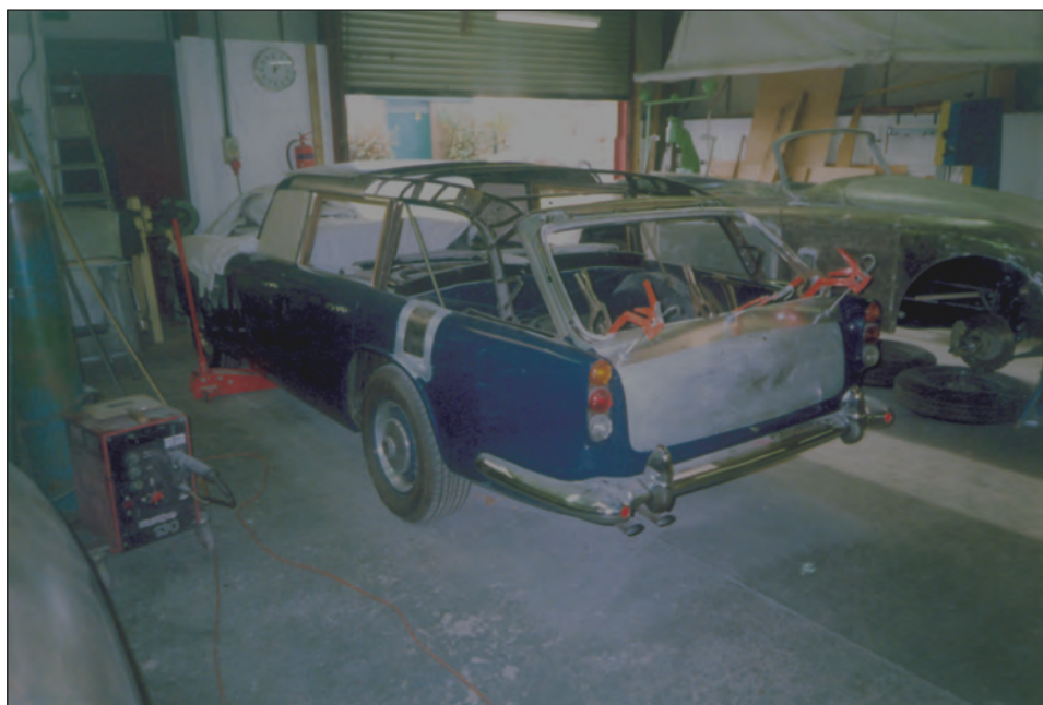
The tubular frame in place and ready for the new panels.
