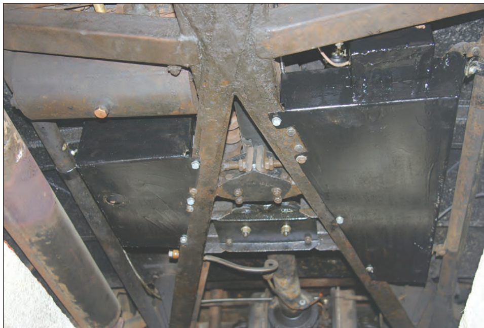
Cover plates neatly fitted to protect the servos.
