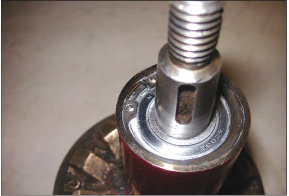
Photo 5, showing the new sealed ball race inside the tube.
