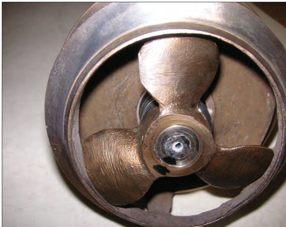
Photo 7, showing the impellor re-fitted on the shaft.
