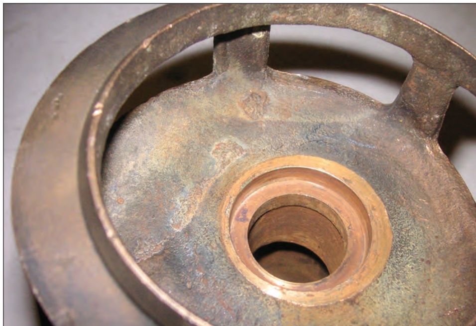
Photo 4, showing the modifications to the aperture for the new gland.
