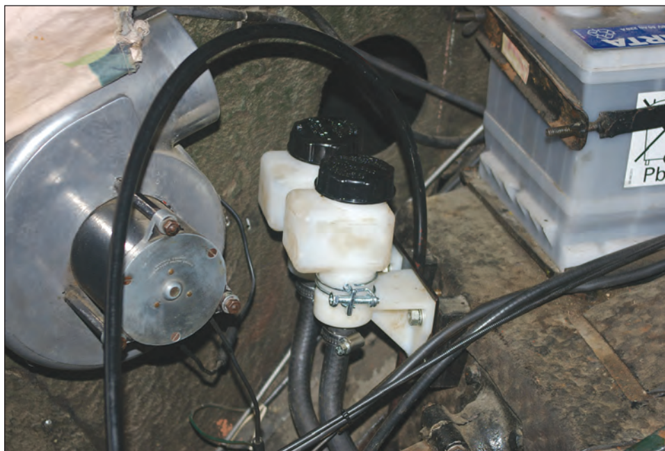
The twin hydraulic fluid cylinders, fitted very neatly.
