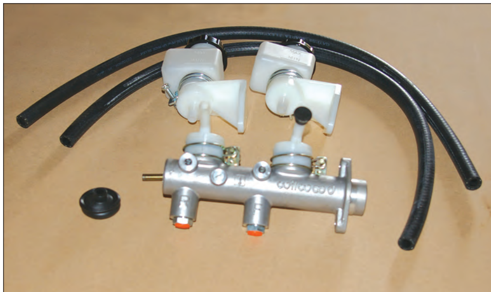
The next seven pictures all refer to the article on page 21. This shows the new master cylinder for the new system.
