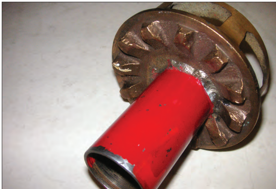
Photo 3, showing the body with new tube attached.
