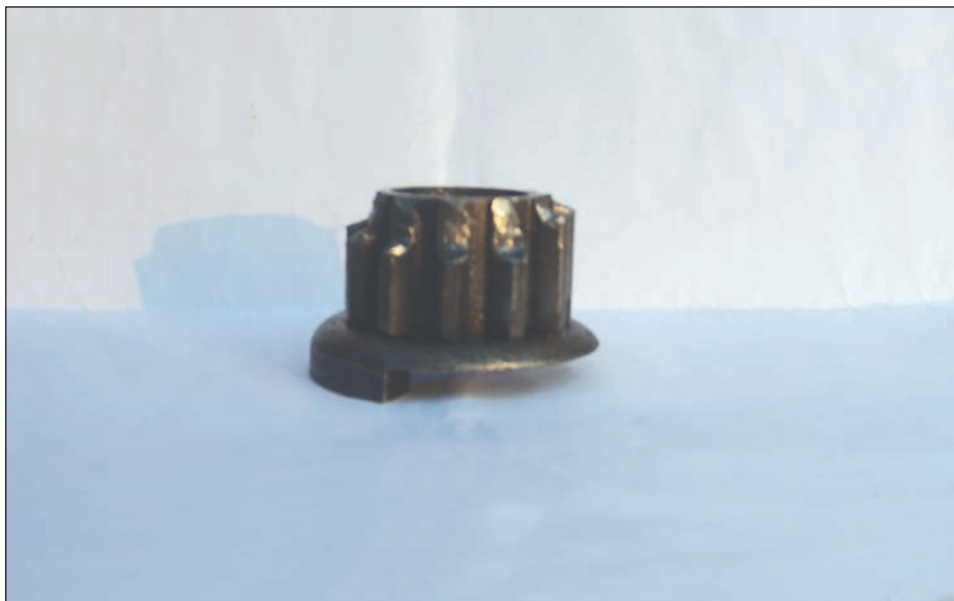
The villain of the piece, Clive's starter pinion.
