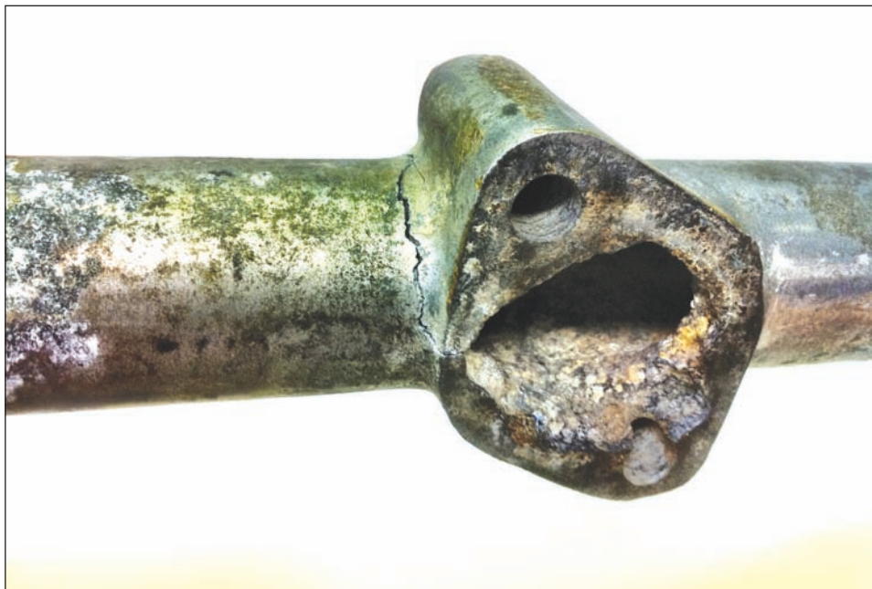
The cracked and corroded water rail on Andrew's engine.
