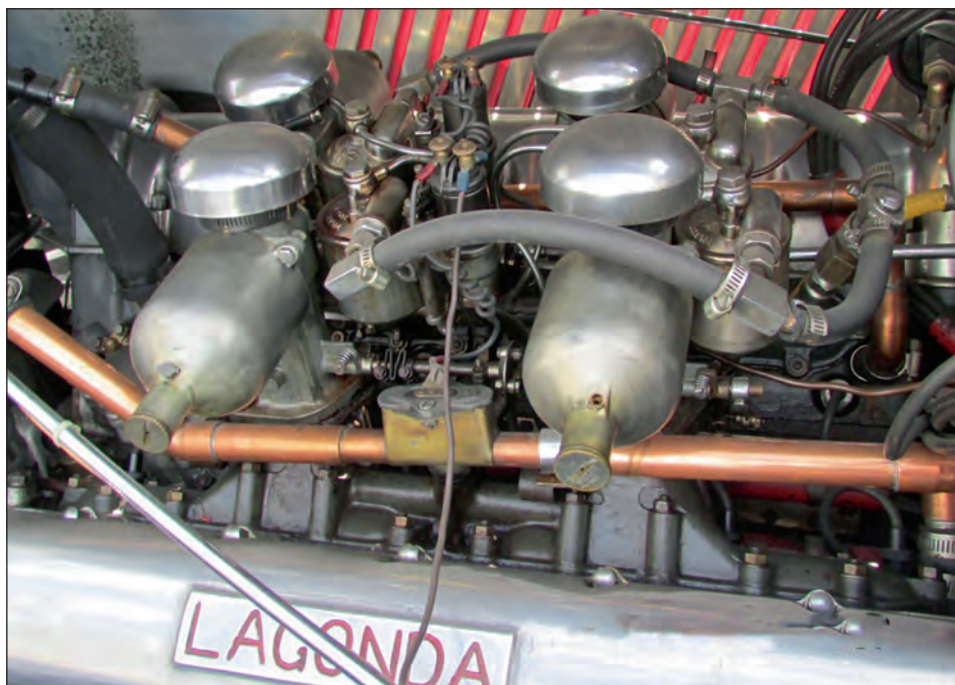
The four downdraught SU carburetors show this engine to be built for performance Pictures copyright to Robert M Lee Trust 2014
