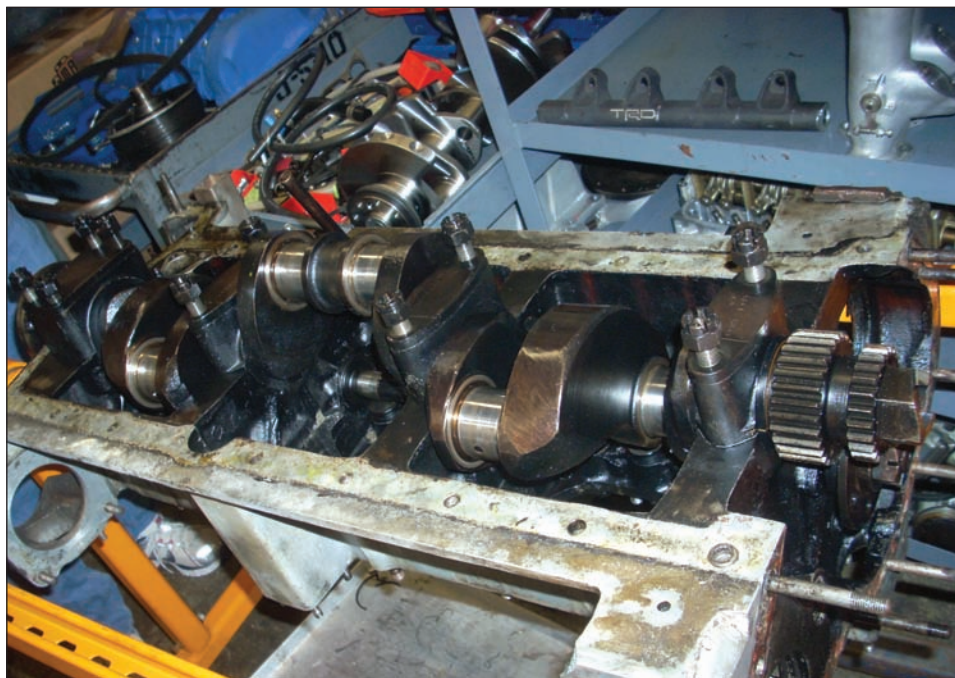
The Invicta engine is stripped for inspection.
