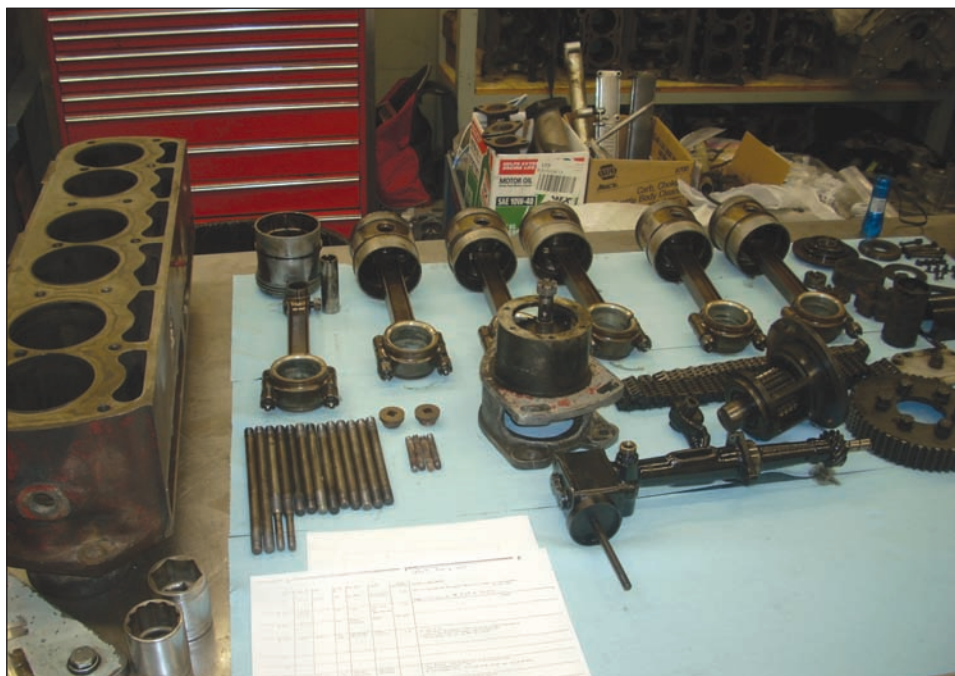
The Invicta engine is stripped for inspection.
