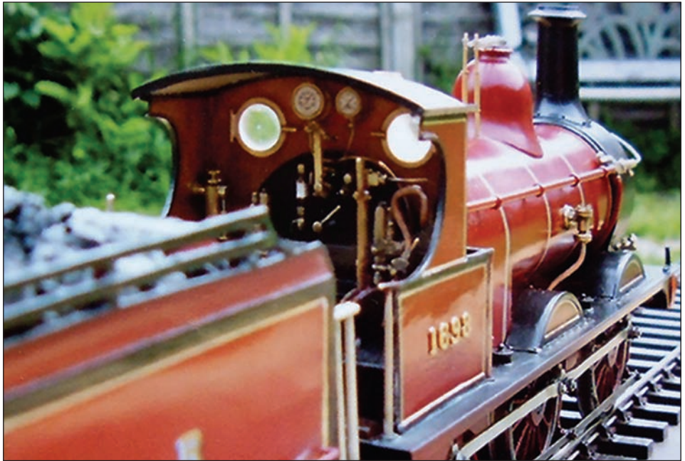
Midland Railway 0-6-0 goods engine, built to "O" gauge
