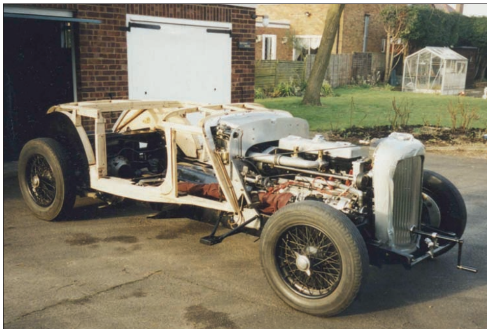
Back home. Body ready for skinning in aluminium
