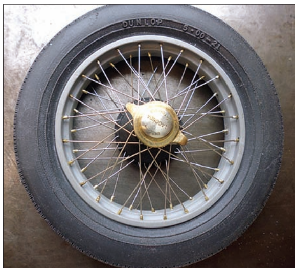
The wheel complete with hub spinner, before painting and plating
