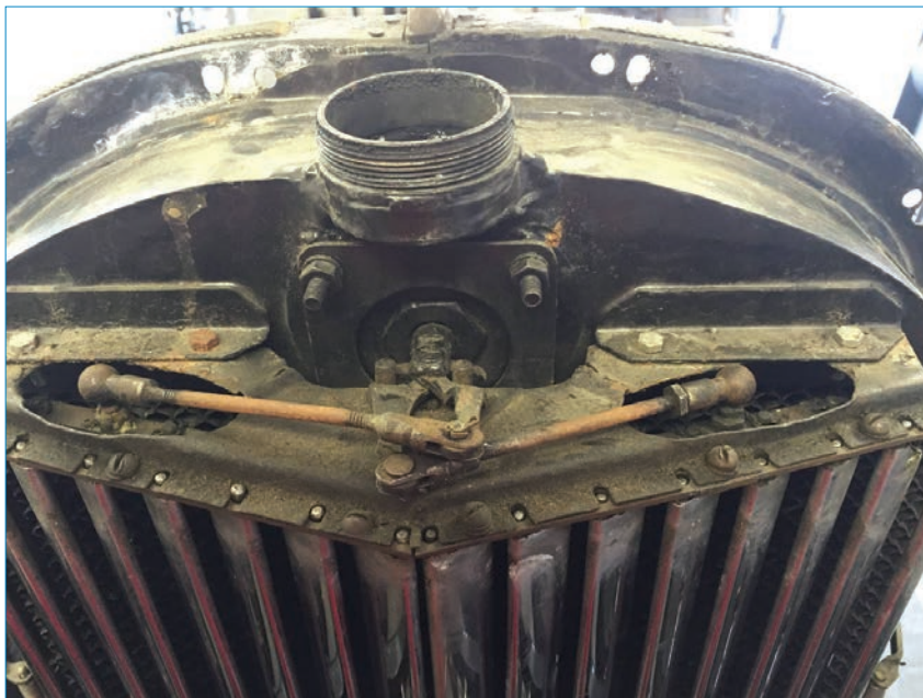
The radiator with the shell removed, showing the operating mechanism for the thermostatically controlled shutters.
