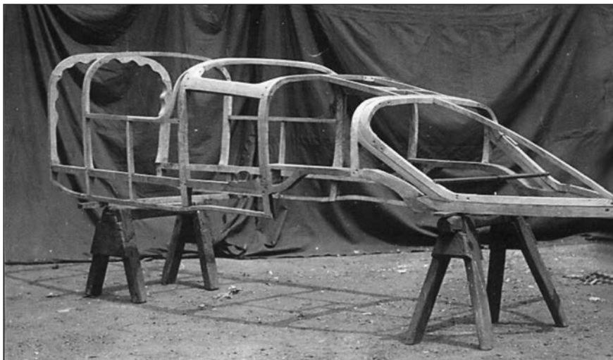
A 1936 Team Car body frame. Picture courtesy of Angela Pugh
