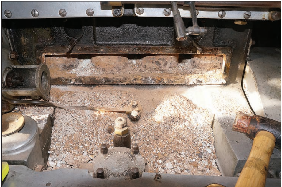
The engine side plate repairs in progress after years of corrosion and scale.
