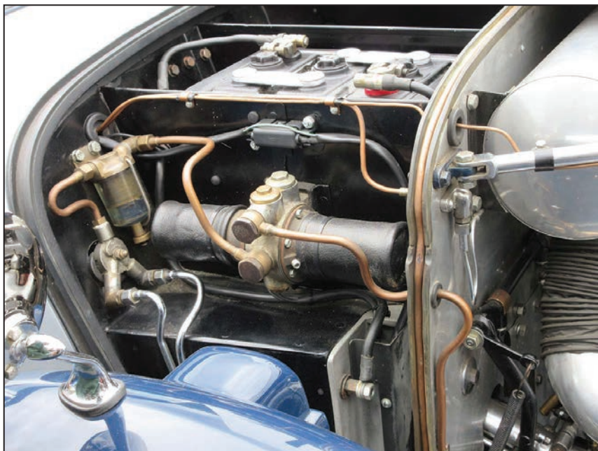
On the LG45DHC/Tourer the pump is behind a shield on the bulkhead
