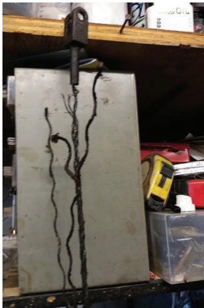
This 14/60 has a cable from the brake pedal to the Compensator box (later cars have a rod). So no rear brakes at all if it snaps!
