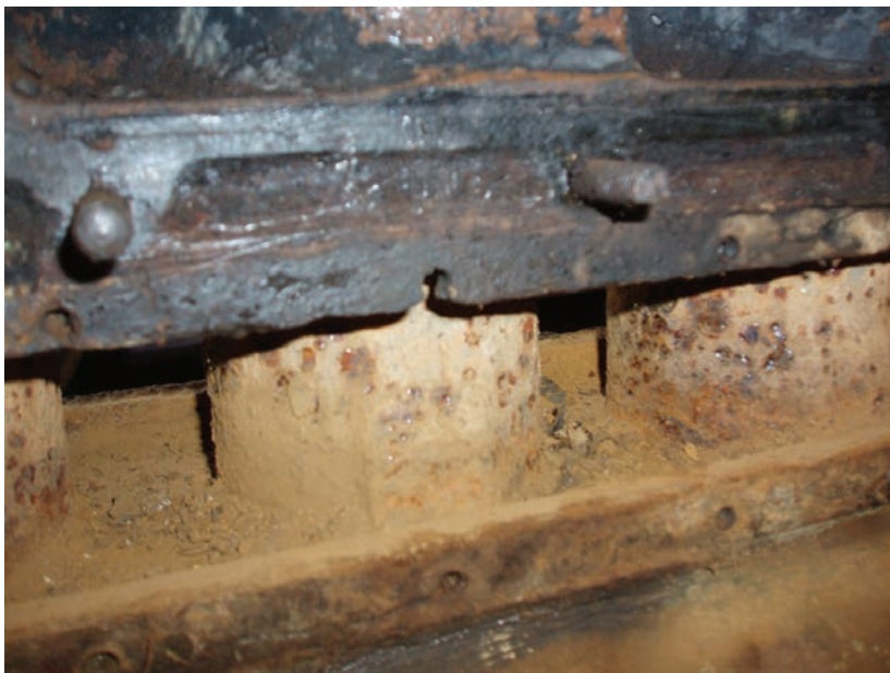
The damage to the nearside water plate mounting holes.
