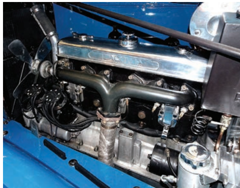
The spotless engine bay - note the twin Vertex Magnetos
