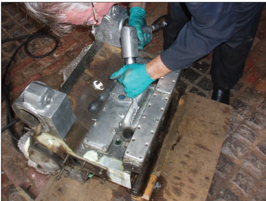
Crack repair behind exhaust manifold
