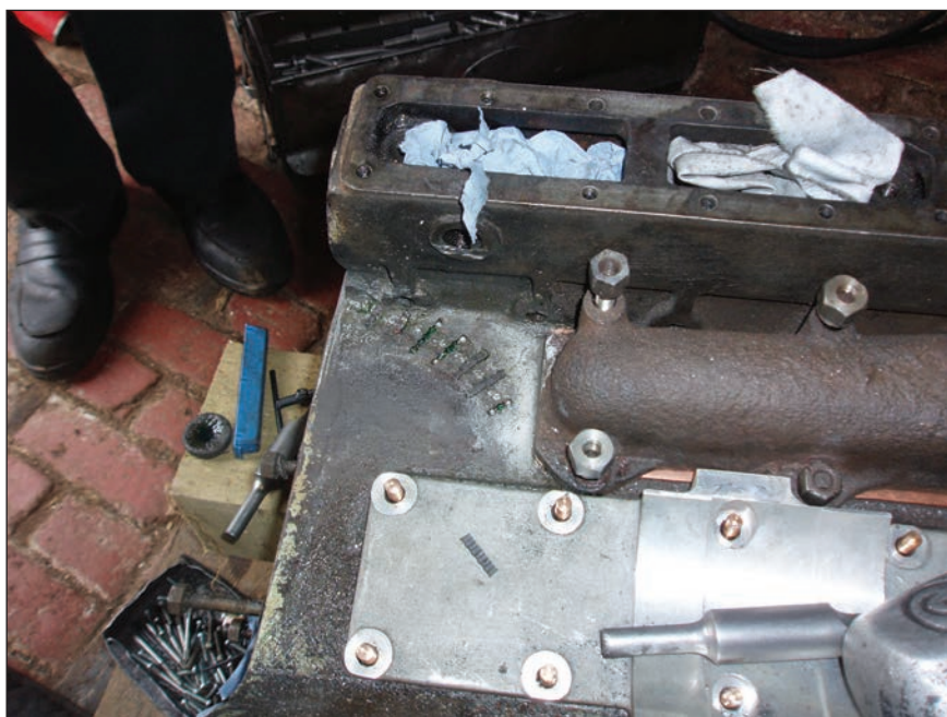
Nearside water plate mounting repairs
