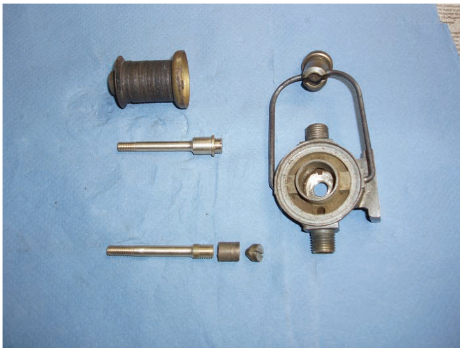
Zenith Fuel Filter, showing repairs made
