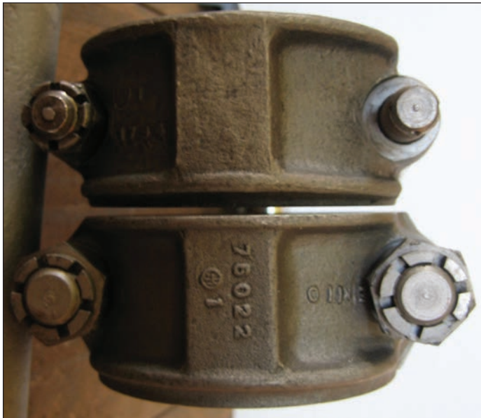
On the top, the original “Vantage” rod for the 2.6 Litre engine, and on the bottom how the big-end was offset to match the offsetting of the 3 Litre cylinder liners. It also shows the increase in the diameter of the integral bolt, found in some later 3 Litre engines and as standard in the DBA engine fitted to the Aston Martin DB2/4MkIII.
