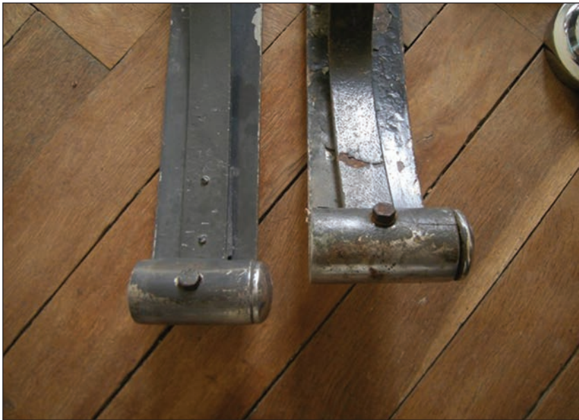
Prior to dismantling - note crack in the right-hand bumper, which Laurence discovered had been expertly repaired inside.
