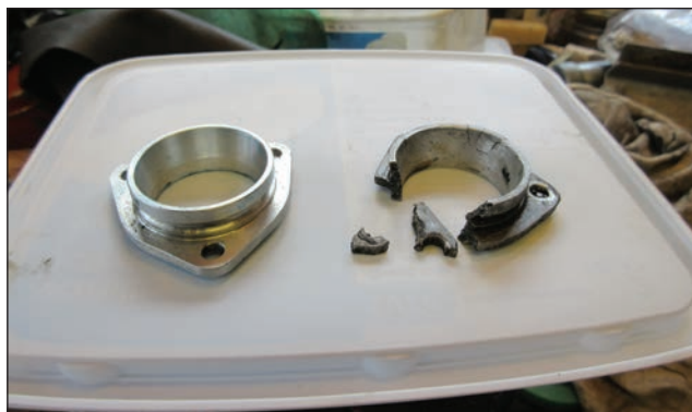
New component (part no. BRK 417) against the old component
