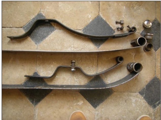
The dismantled bumpers showing all the components.
