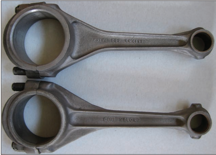
Two connecting rods showing the substantial change from the original W.O. design with white metal bearing, on the bottom, to the “Vantage” design with thin-wall shell bearings to handle the significant increase in power, on the top.
