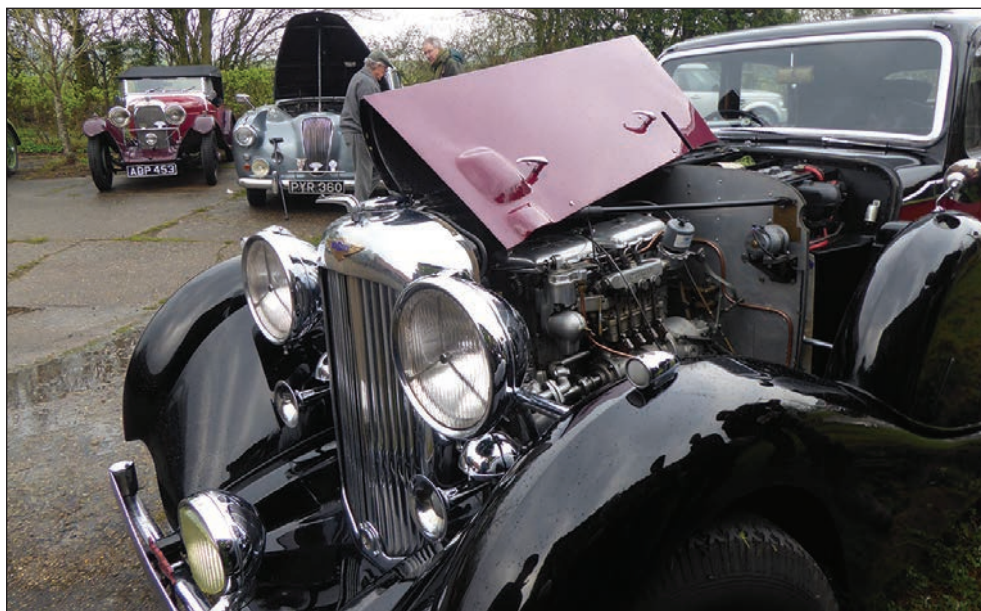
The Gardner diesel engine in John Hutchby's LG45
