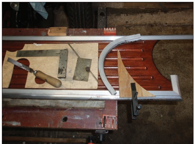
The jig for forming the rear edging curve and the result
