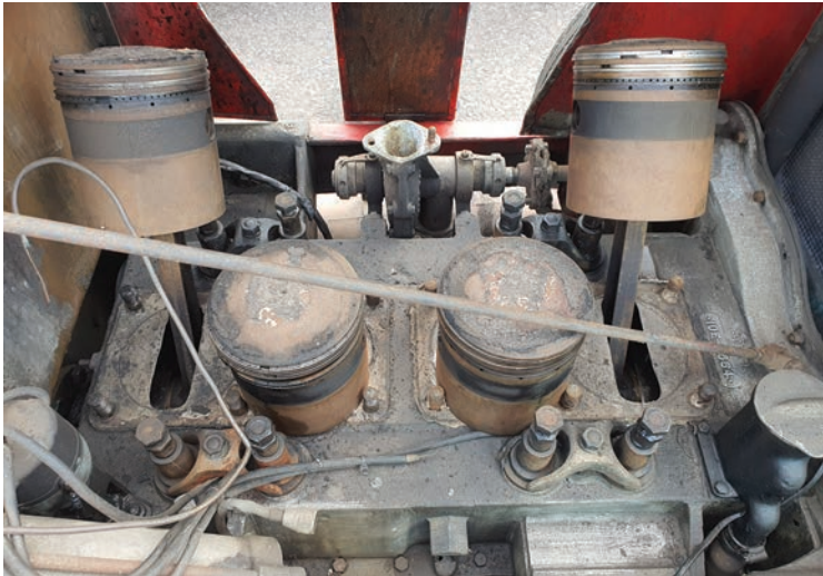
Another Beaulieu spot - the insides of a 1913 American LaFrance engine. 9.7 litre four cylinder - there's no replacement for displacement!
