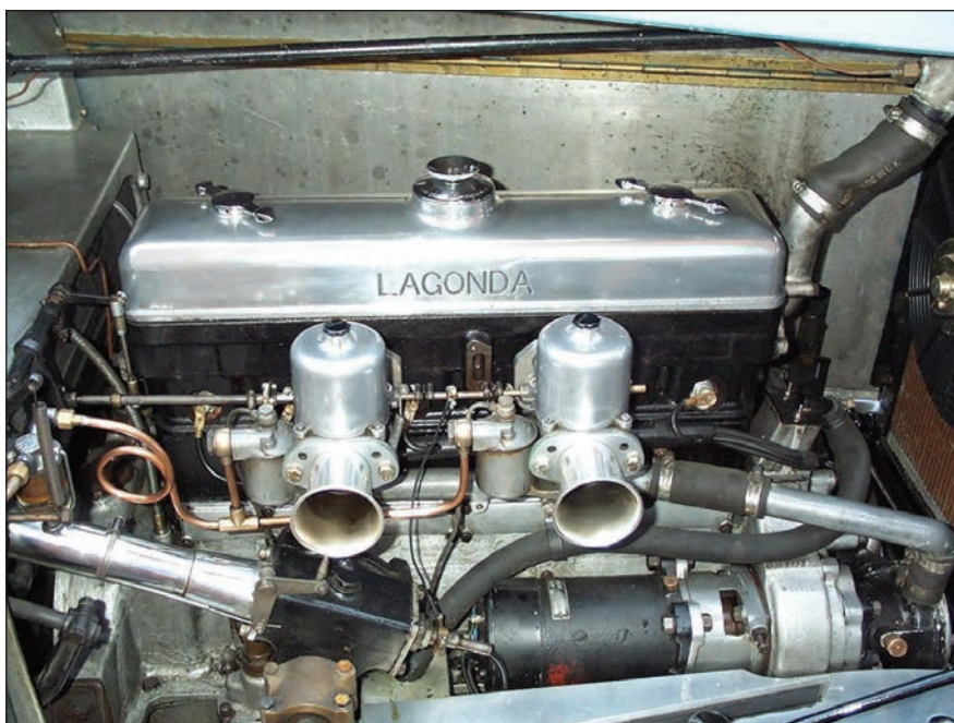
The engine of 'Wotsit', fitted with Jaguar SU Carburettors
