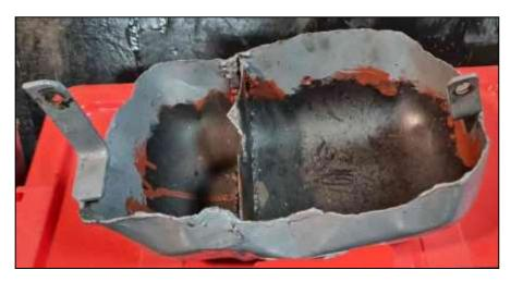
You might want to study this image momentarily, prior to making a decision to invest. It works by being firmly secured to the rear of the lower bell housing, as it were, by the two cleverly fabricated brackets that locate on bolts selected at random from the rear of the engine. A sump plug is incorporated into the pan to drain this superbly designed device. It is easy to recognised skilled workmanship and finish in this prototype.
