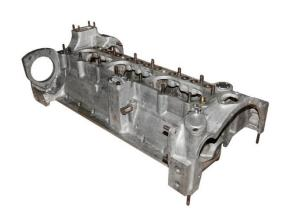
Original Invicta crankcase, fully crack tested and pressure tested, with certificates. Suitable for M45s, but it does not have the improvements in the casting alloy, main bearing arrangements, and bolting arrangements to the block that were introduced by Lagonda for the M45R and LG models.
