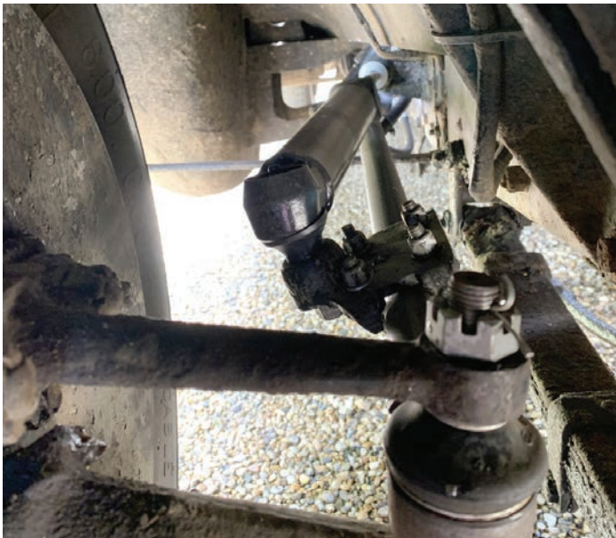
From the front of the car - the hydraulic ram attached to the draglink
