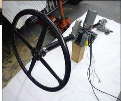
Right: Steering column with EPS ready to install
