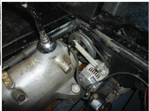
Below right: Alternator general arrangement
