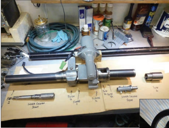
Top: Steering column for EPS under construction
