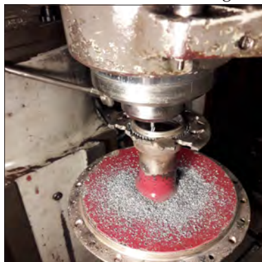
Removing the broken outer spoke ring
