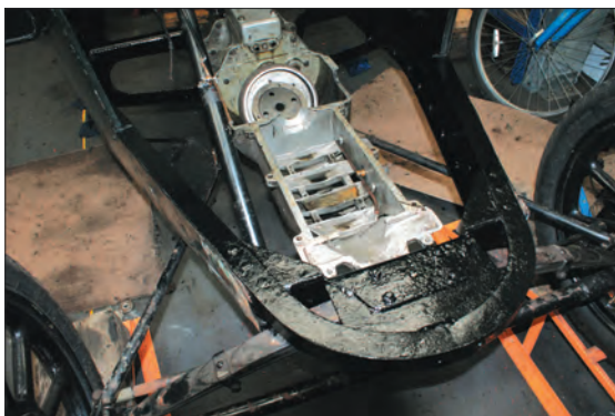
The sump, clutch housing & gearbox are a single aluminium casting.
