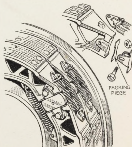
Pull-off springs and shim method of adjustment for the rear brake shoes.
