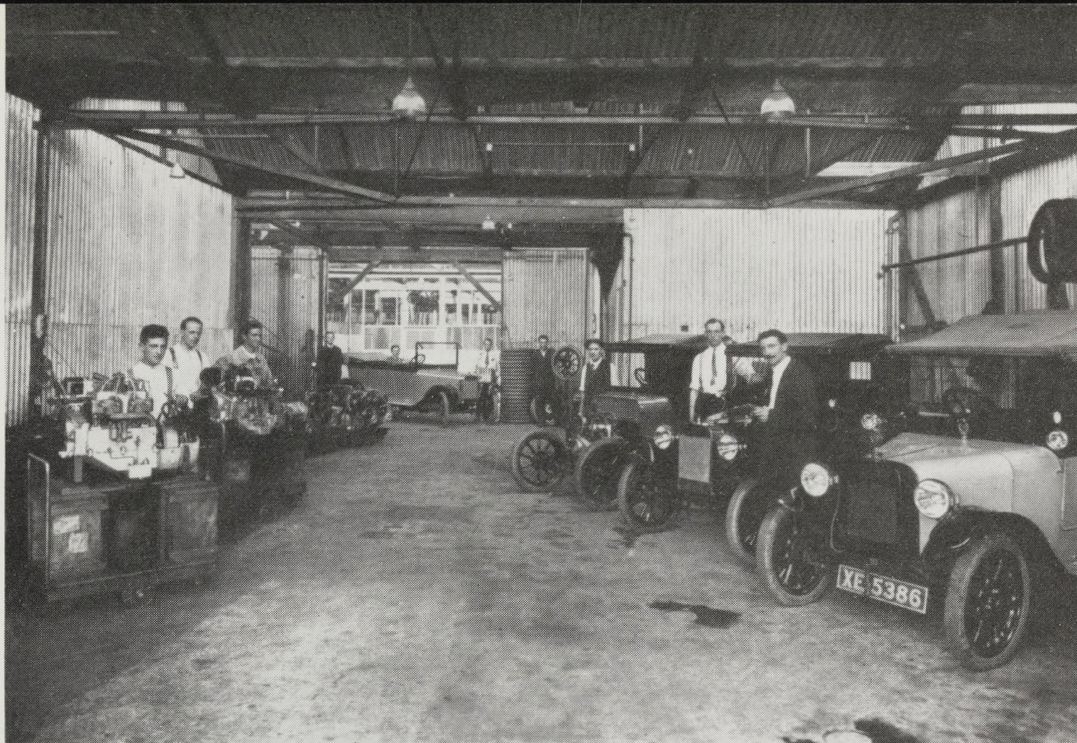
Factory view of late 11.9s during period of maximum production about 1921-2. Engines are being tested on left, car ready for delivery on right.
