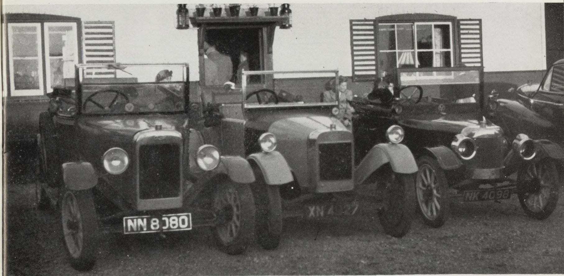
Three Lagonda light cars showing three distinct radiator types and general increase in weight. (L. to R.: 1924, 1923, 1914 now owned by Marcia Fisher, Nancy Audsley and C. Elphinstone.)
