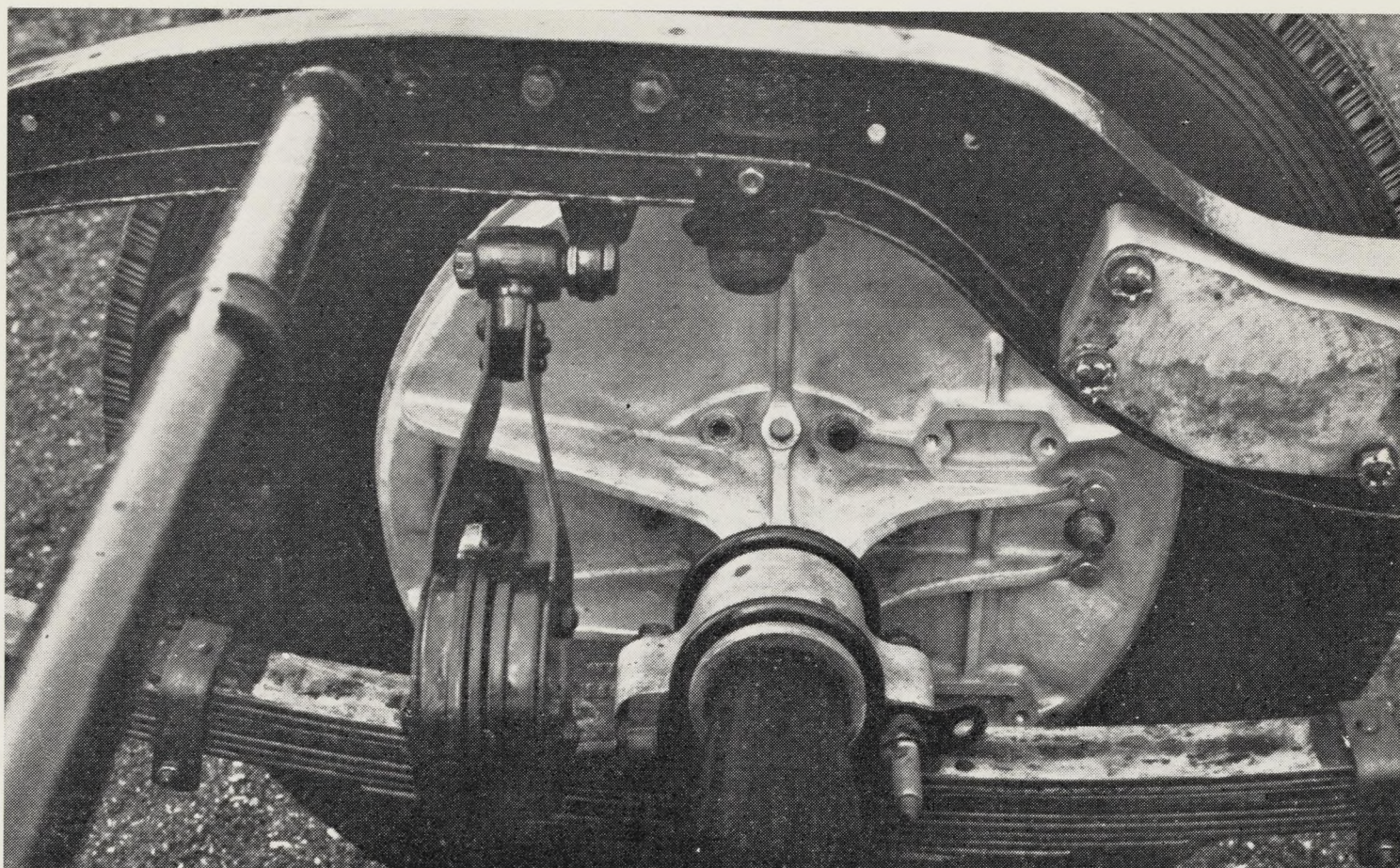
Rear axle (near side) during re-assembly
