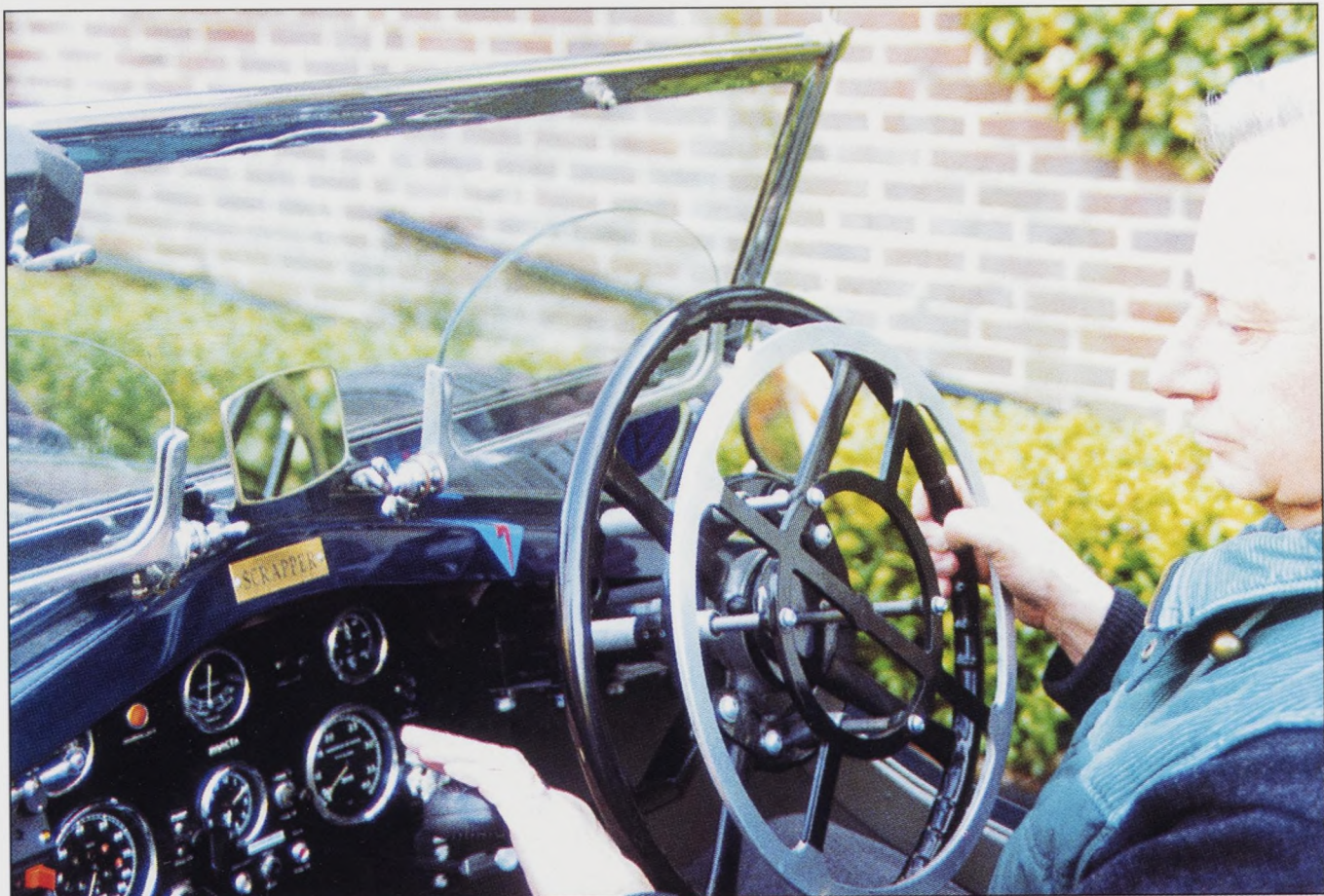
Michael demonstrates the accelerator ring, operated with the right hand and the control for the brakes with the left hand.
