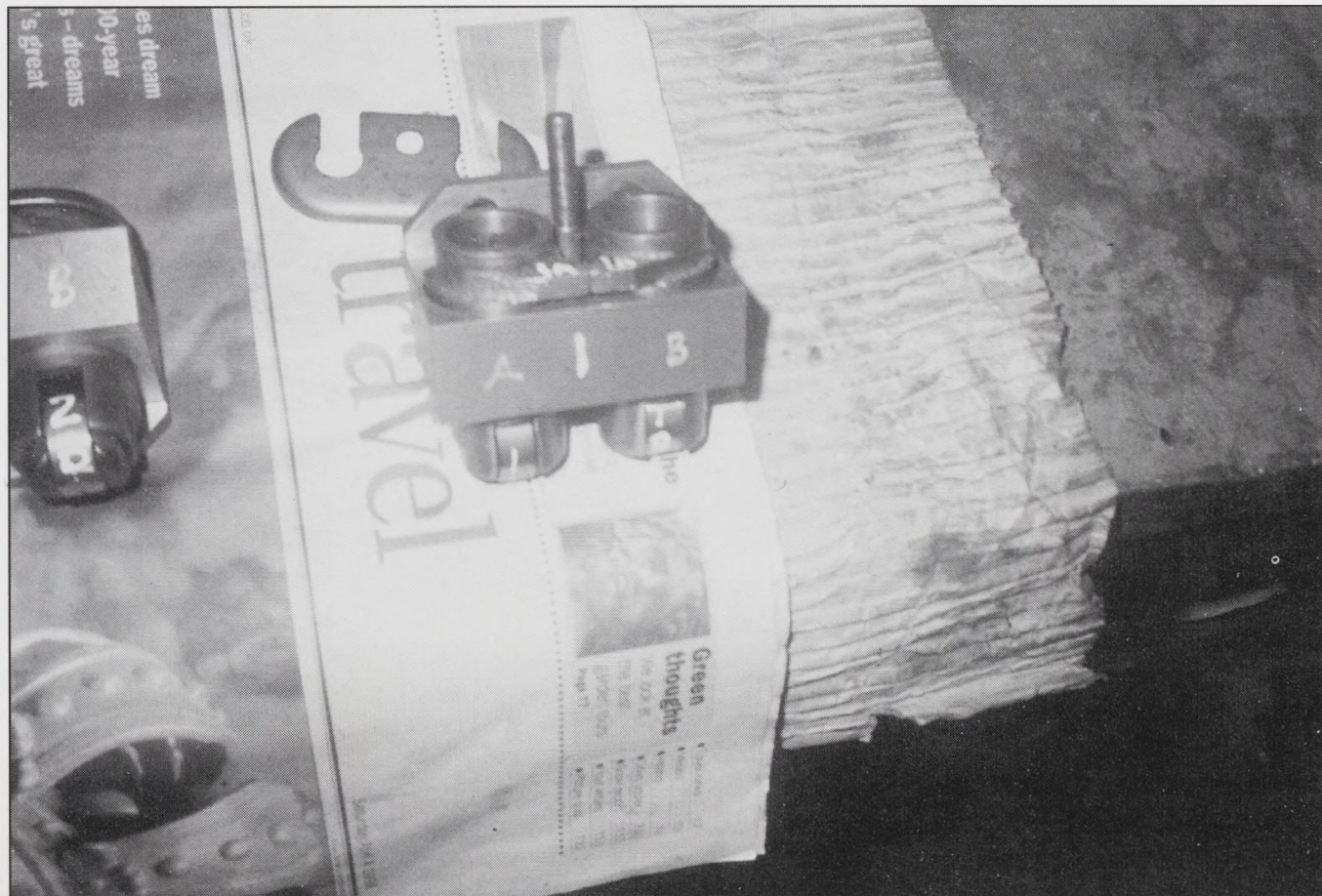
Carrier block complete with sleeves and roller follower inserts.
