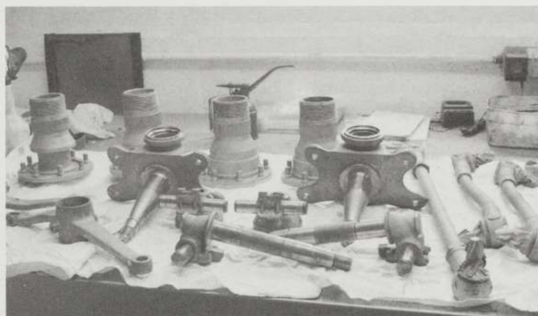
A small amount of crack testing for V12 front suspension.
