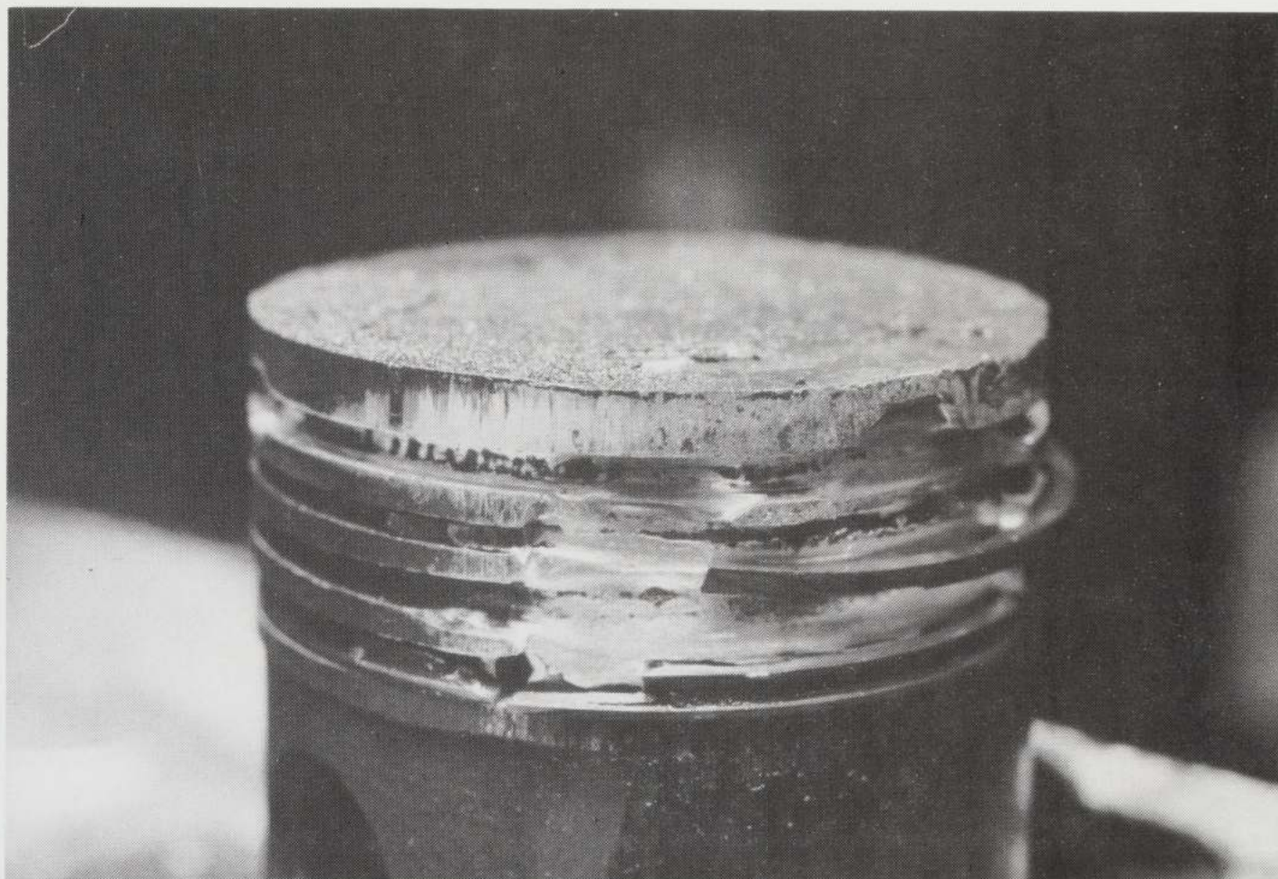
Top: One of the eight broken ringed pistons, compression was somewhat reduced. Bottom: Not a lot of room to work! The tissues are for weeping into!
