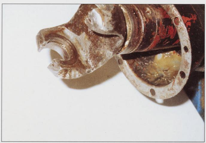
Wear on the shoulder, which, with wear on the spider, gives up to 25mm movement
