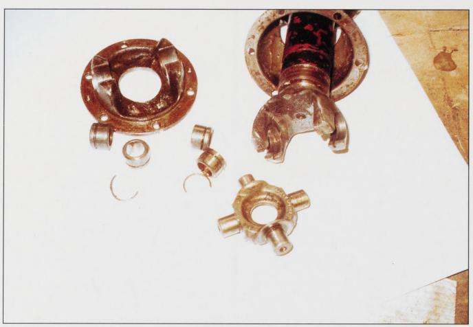
The Spider, bearings and retaining clips
