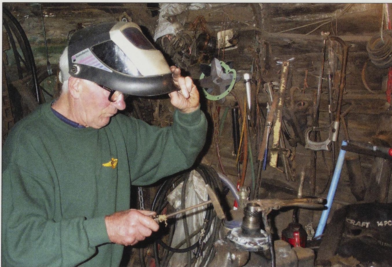
Alan Brown welds Nick Hine's broken drive shaft in a pig farmer's workshop, en-route to Silverstone.
