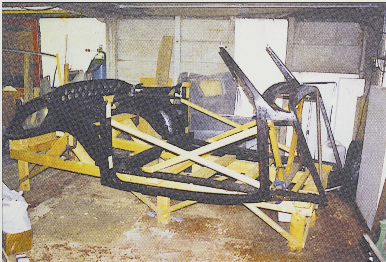
The newly restored body frame takes shape
