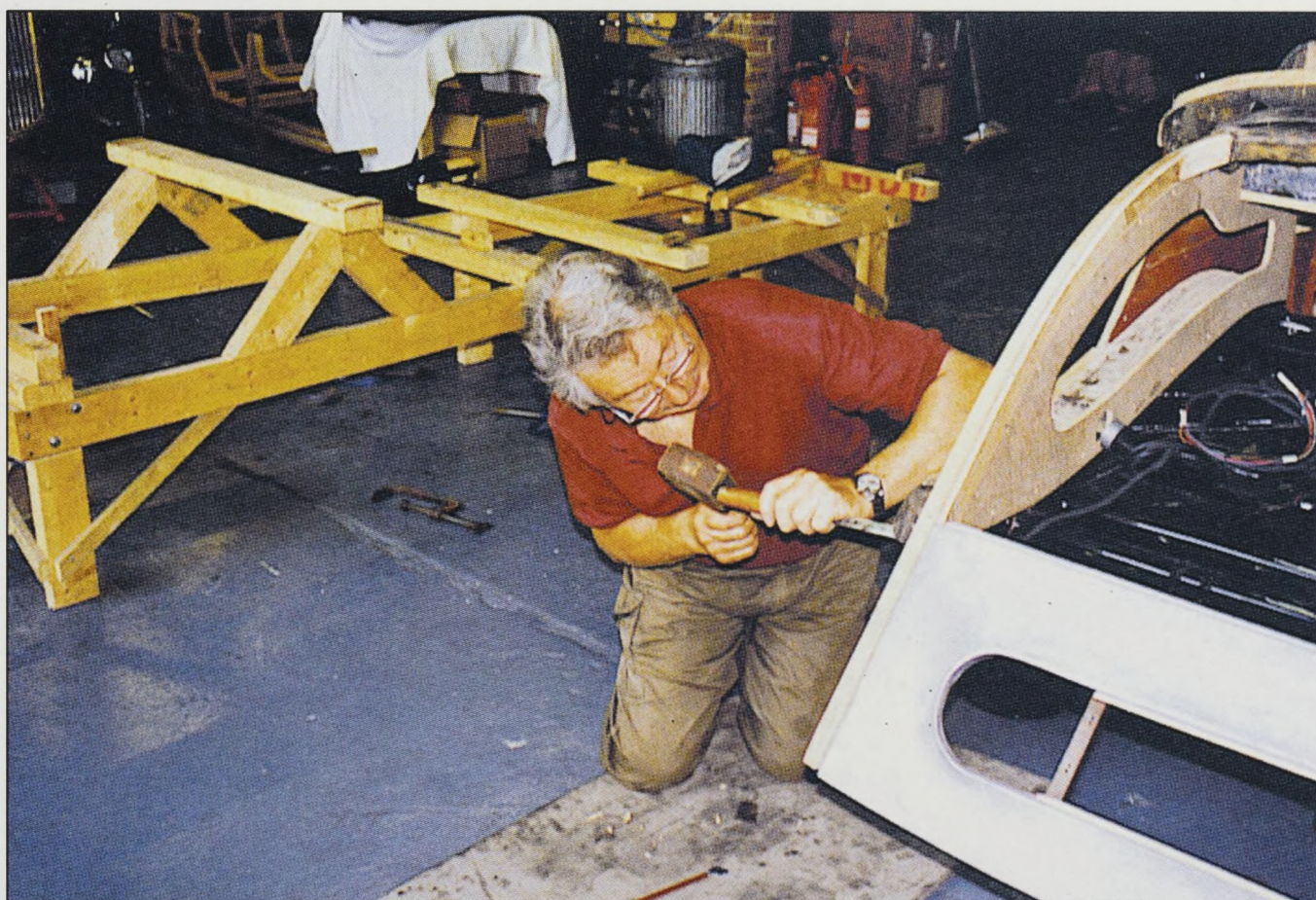
Dennis Carter carefully removes the old panels
