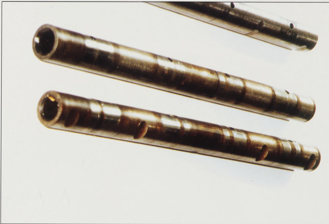
Up to six thou wear on the rocker shafts!
