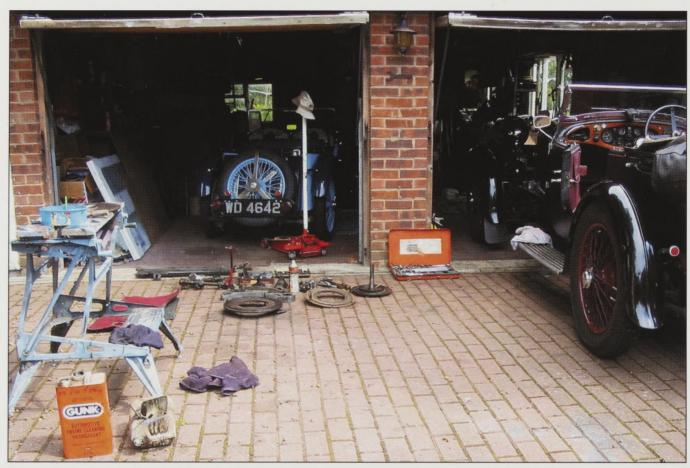
The clutch parts removed ready for inspection.
